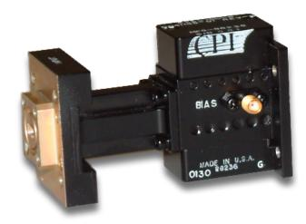
Ka-Band all solid state multifunction component consisting of a bandpass filter, passive limiter, and 70 dB attenuator.
